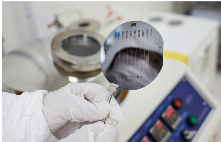
Silicon wafers of thin-film microfabricated electrodes can be implanted into a patient to record from or stimulate the nervous system—the vagus nerve in particular. Image credit: The Feinstein Institutes for Medicine Research.
